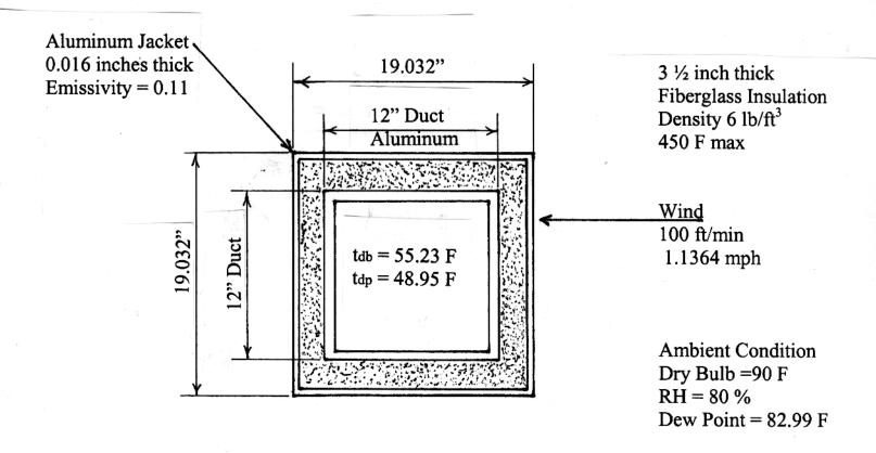
At the end of the duct run the inside duct air dry bulb did not get cooled below the inside duct air dew point therefore the inside duct air is not condensing. To determine if the inside duct surface temp. is below the inside air dew point would require another computer analysis at the end of the duct run.
